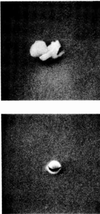
Fig. 21—SEM micrographs showing particulate agglomerates on the surface (A) and in a micropinhole (B) of a sprayed-on \text{TiO}_2 film. Vertical measure of top defect is 1.8\ \mu\text{m} and of bottom defect is 0.6\ \mu\text{m} .
